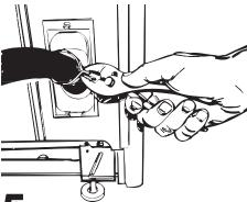
Place hose clamp over washer drain connector. Push drain hose onto washer connector. use pliers to open clamp and slide clamp over drain hose. Check for good fit.
